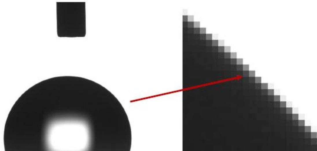
Fig. 13: Image of sessile drop with more change range of sharpness used common Background light and lens.
