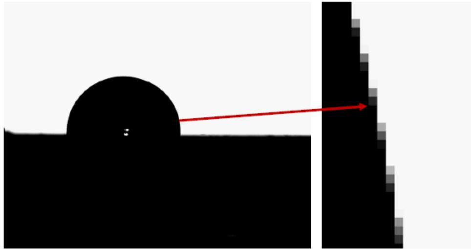
Fig. 12: Image of sessile drop with little change range of sharpness used Parallel light Background light and telecentric lens.
