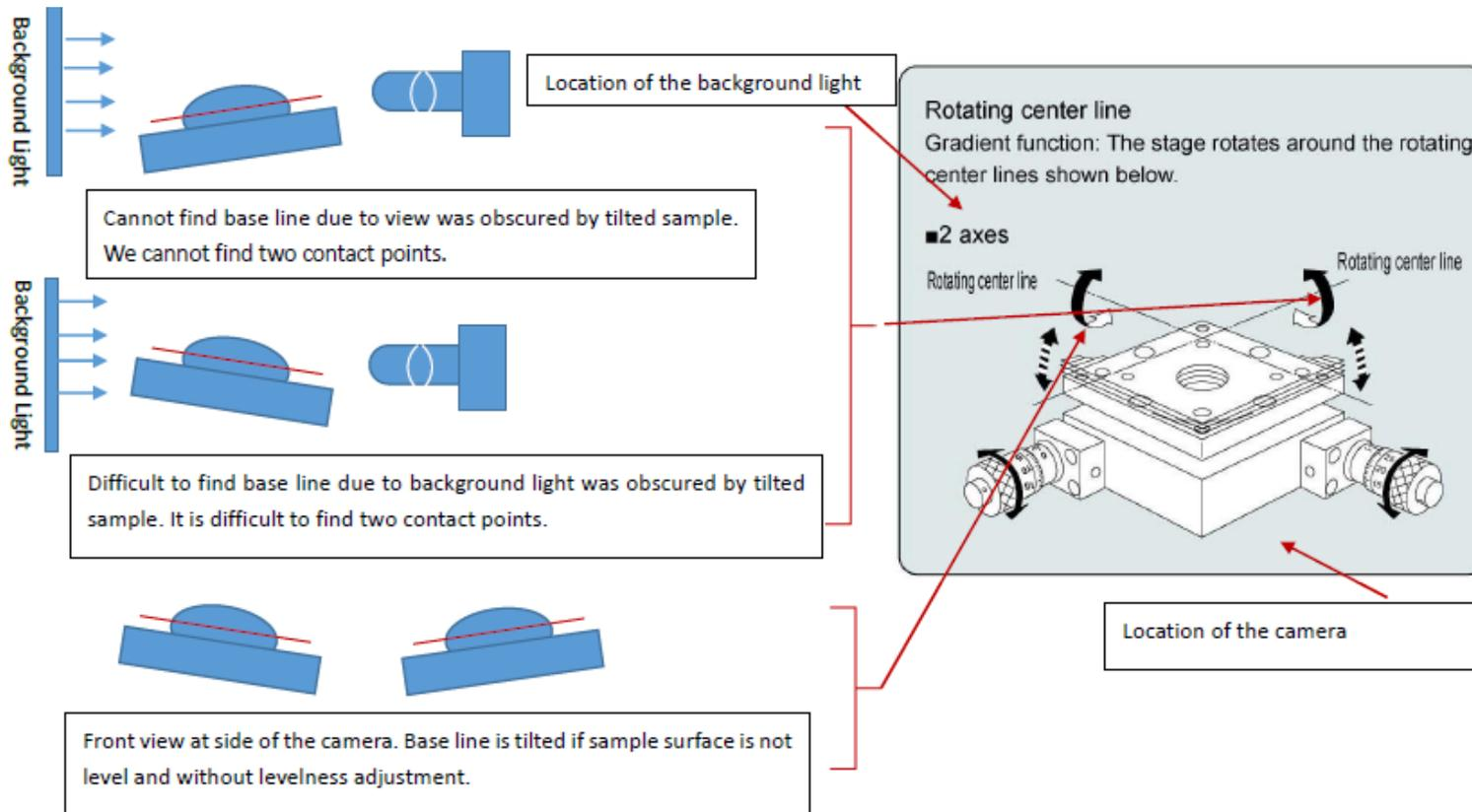
5, Tilting system for measurement of roll-off angle of KINO’s contact angle meter adopts motorized rotation stage with very low backlash, low wobble (about 40urad) and high absolute accuracy (about  $0.01^\circ$  ). KINO exclusively provides you specially designed mechanical Structure (Rotating only Lens, sample stage and its control system)
