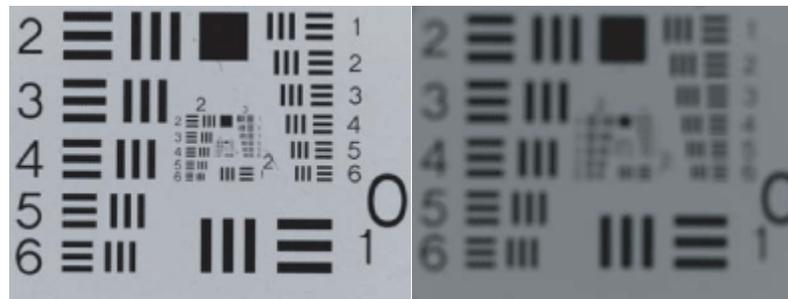
Fig. 7: good and bad contrast achieved with optics of varying CTF looking at a standard USAF test pattern.
