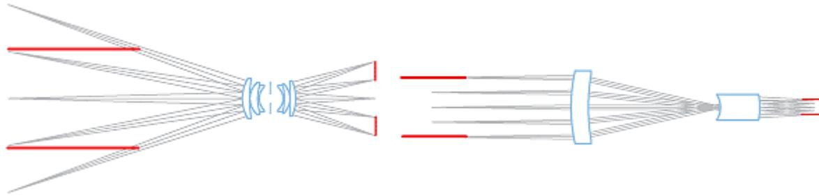
Fig. 6: Common optics (left) project longitudinal geometrical information onto the detector, while telecentric lenses are not.
