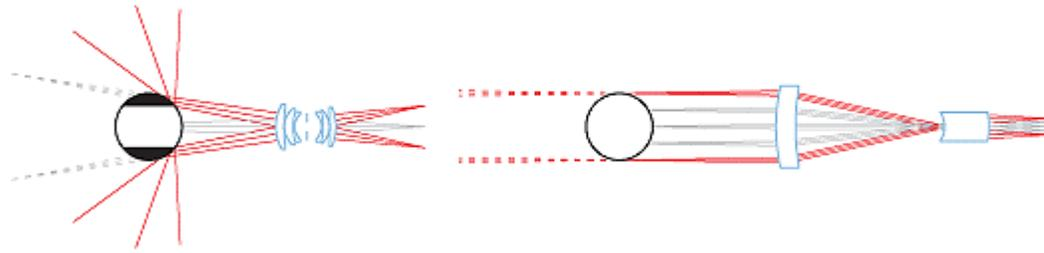
Fig. 8: Border effects in a common imaging lens are strongly reduced by means of a telecentric lens
