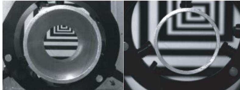
Fig. 5: Common optics showing significant image perspective error (on the left). A telecentric lens is able to cancel any perspective effect (on the right).
