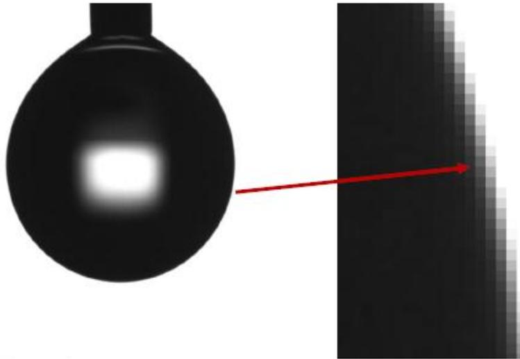
Fig. 11: Image of pendant drop used common Background light and lens. We can find more change range of sharpness at image edge when zooming it about 1500X.
