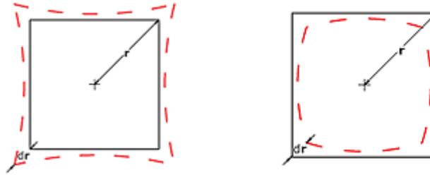
Fig.3: “pincushion” type distortion “barrel” type distortion
