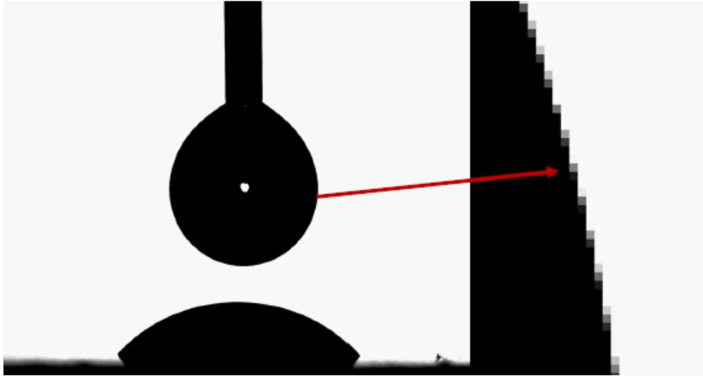
Fig. 10: Image of pendant drop used Parallel light Background light and telecentric lens. We can find little change range of sharpness at image edge when zooming it about 1500X.
