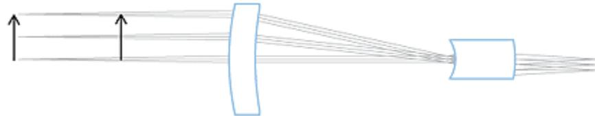
Fig. 2: in a telecentric system rays get into the optics only with an almost parallel-to-the-axis path.
