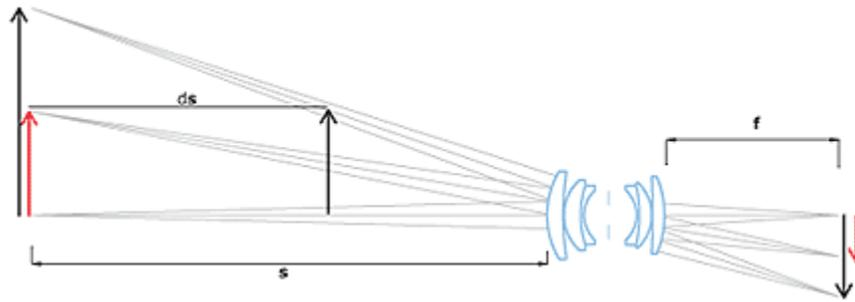
Fig. 1: a standard lens generates different size images when changing the object-to-lens distance (indicated as "s" in the drawing). On the other hand, objects of different sizes would look as if they had the same dimensions, provided they subtend the same viewing angle.
