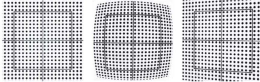
Fig. 4: on the left an image of a distortion pattern taken with a telecentric lens, where no radial or trapezoidal distortion is present. In the middle the image of the same pattern showing strong radial distortion. On the right an example of trapezoidal distortion.
